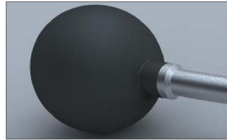
Figure 2: Ionization Chamber IC [7]
