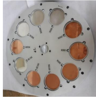
Figure 3: 10 position filter wheel NS- series 30 to 300keV
